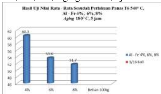
Gambar Grafik 4.4. Nilai Rata – Rata Sesudah Perlakuan Panas T6 540° C, Al – Fe 4%, 6%, 8%, Aging 180° C, 5 jam
