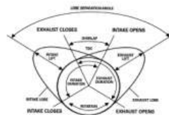
Gambar 2.8. Diagram lobe separation angle
