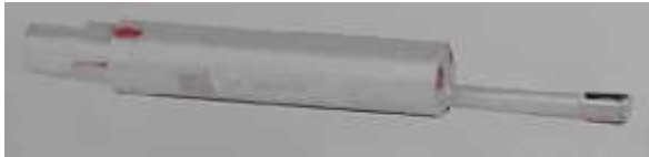
Gambar 5. Stylus Surface Roughness Tester
