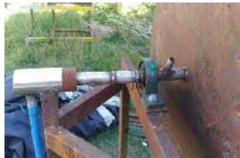
Gambar 4. Penampang Bearing house output dan Bantalan
