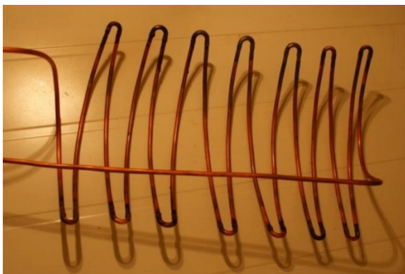
Gambar 4. Heat Exchanger Tipe Serpentine
