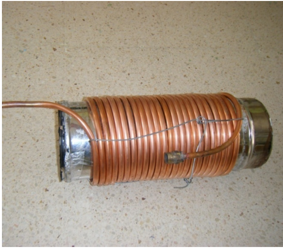
Gambar 2. Heat Exchanger Tipe Helical
